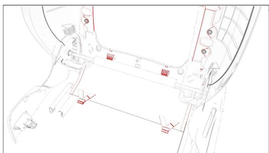
3. Release the clips that attach the shell apron to the underside of the seat, and then remove the shell from the seat.
