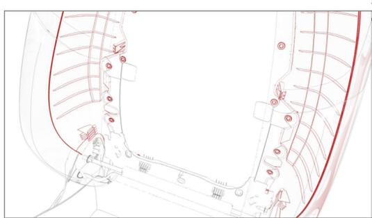
2. Release the clips that attach the seat back shell to the driver seat, lift up on the shell to unhook it from the seat back frame, and lay the shell back.
