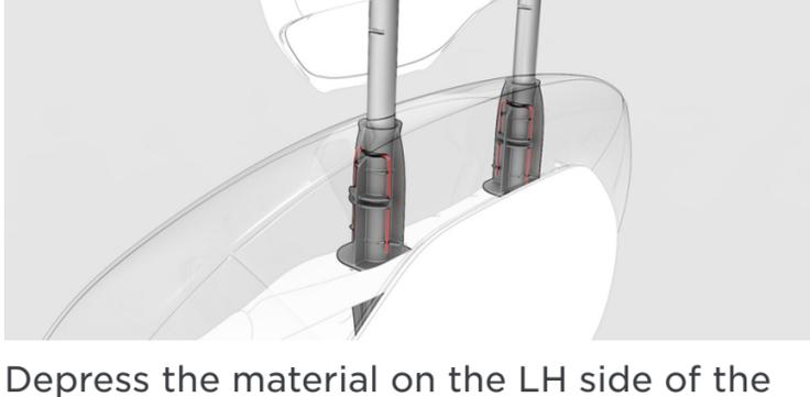
5. Depress the material on the LH side of the inboard headrest post (under the headrest) to expose the retaining spring that restrains the post into the driver seatback.
